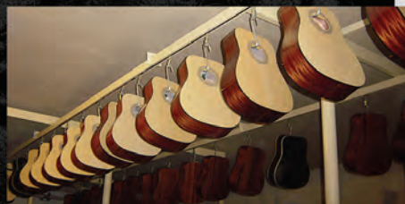
Finished acoustic bodies travel through an air-filtered drying room.
