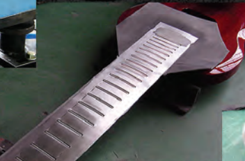
To avoid fretboard damage, this innovative jig provides protection during fret dressing.
