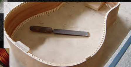
Kurling is attached to the body rim by hand.
