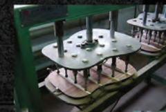
Hydraulic presses hold back bracing and body rims in place.
