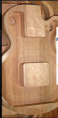
CNC machines make for precision routing of this Kat body. Note the quality of Mahogany.
