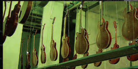
These highly flamed Les Paul Standards make their way through the drying room.
