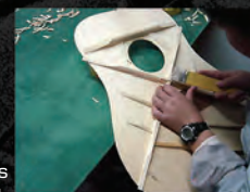
Skilled hand work shapes acoustic guitar bracing.
