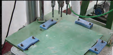
"Gang" drill presses with multiple heads ensure proper placement of holes. In this case LP control holes.
